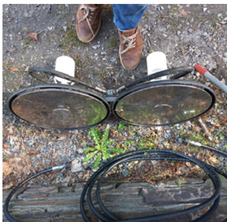
A hand controlled two-disc power washer was used to clean the Smoltscreen weekly.
